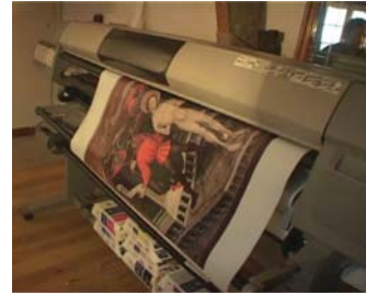
Figure 8. Papelgel material being printed in a HP Designjet 5500 as any other conventional photo media
