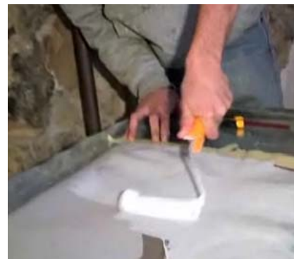
Figure 9. Papelgel printed side is glued to moisten it and later on transfer the ink layer on top of the machined
