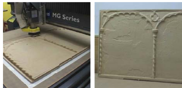
Figure 6. Milling process and table sample
